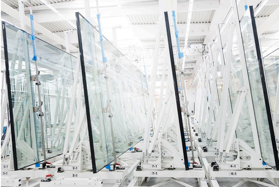
caption: [24-10_01]: On the new insulating glass production line, sedak manufactures insulating glass in formats up to 6 meters in sedak tempered+ quality.
